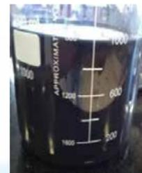
Sludge as received – No Flocculant
