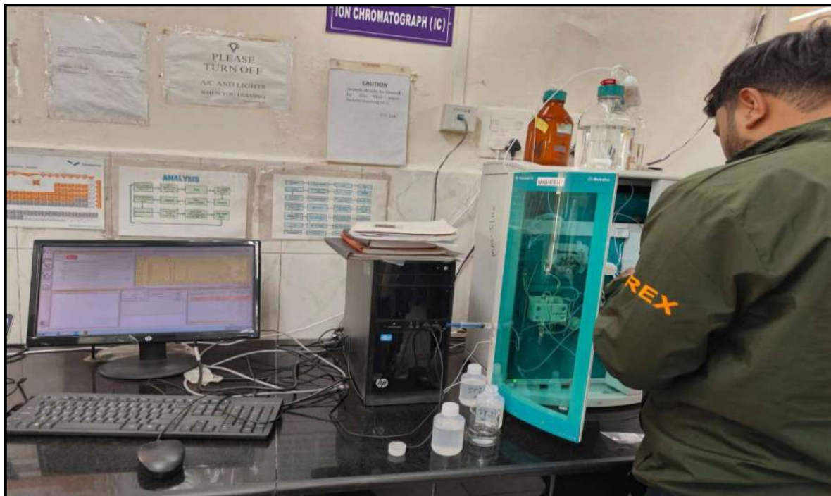
Figure 3.3: Measurement of ions in the collected water samples using Ion Chromatography (IC)
