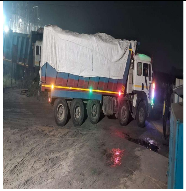
Pond Ash Hywa Fully Covered with Tarpaulin Sheet
